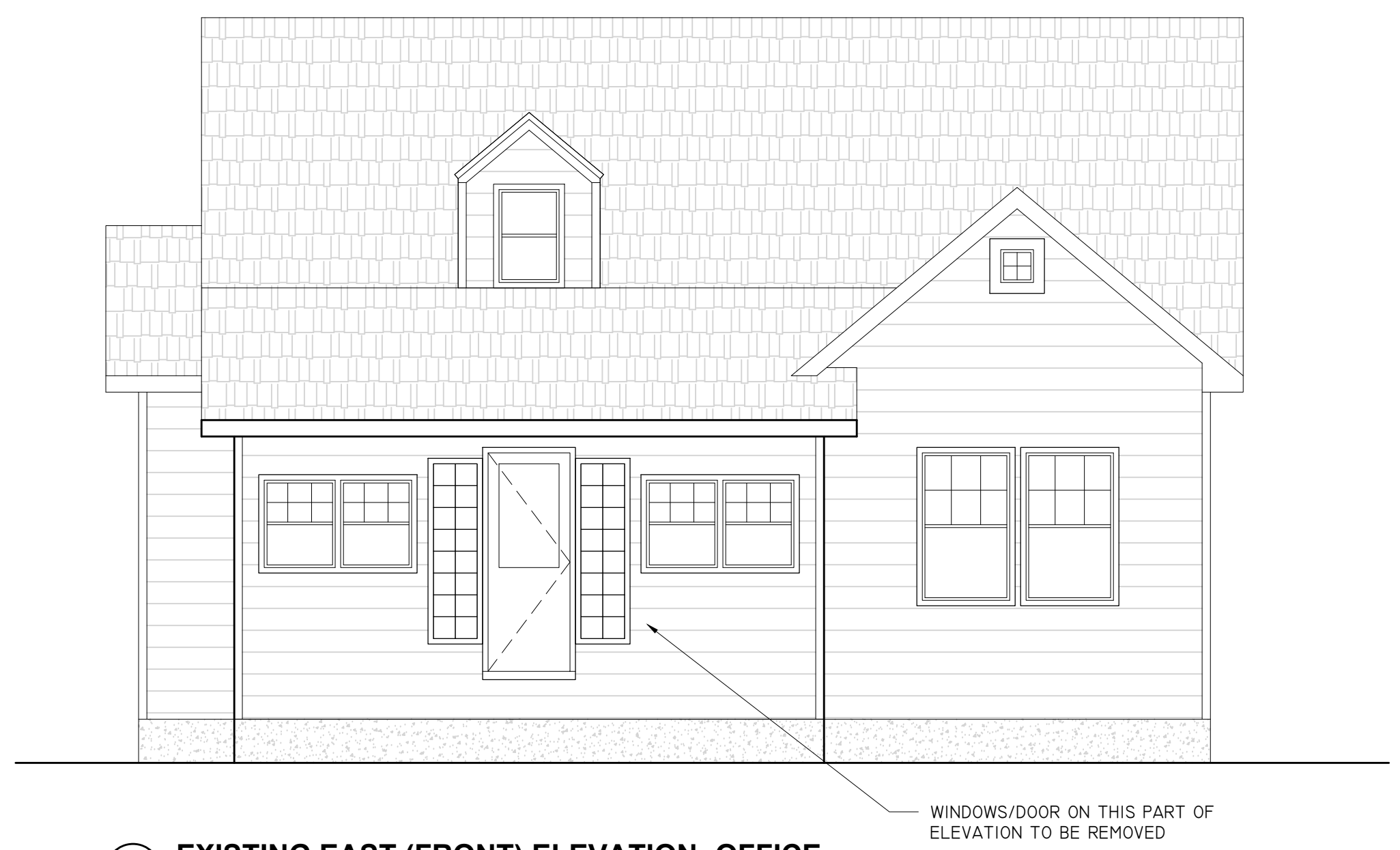
1 A601 EXISTING EAST (FRONT) ELEVATION- OFFICE SCALE: 1/4" = 1'-0"
